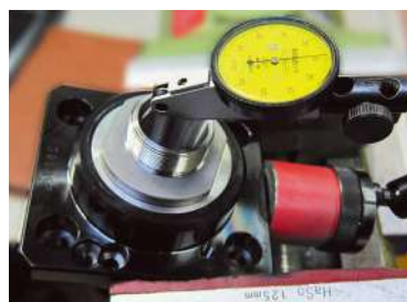
Output End Inspection
